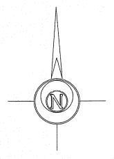
Horizontal Datum is based on the Wisconsin State Plane Coordinate System Grid, South Zone, all bearings are referred to Grid
